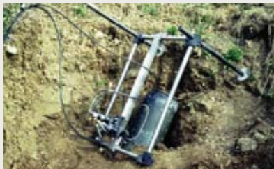
Cutting a burn out hole with 3-Axis Cutting Table
