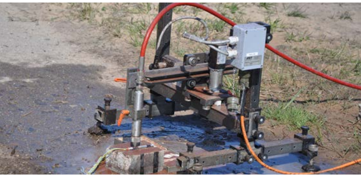
Cutting a detonator with a 2-axis cutting table
