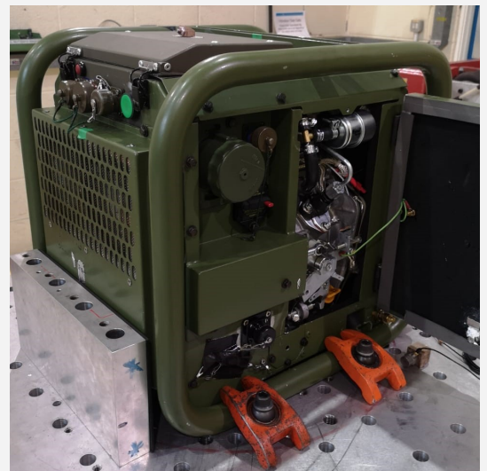
On & off road shock & vibration for wheeled & tracked vehicles to Def Stan 00 35.
